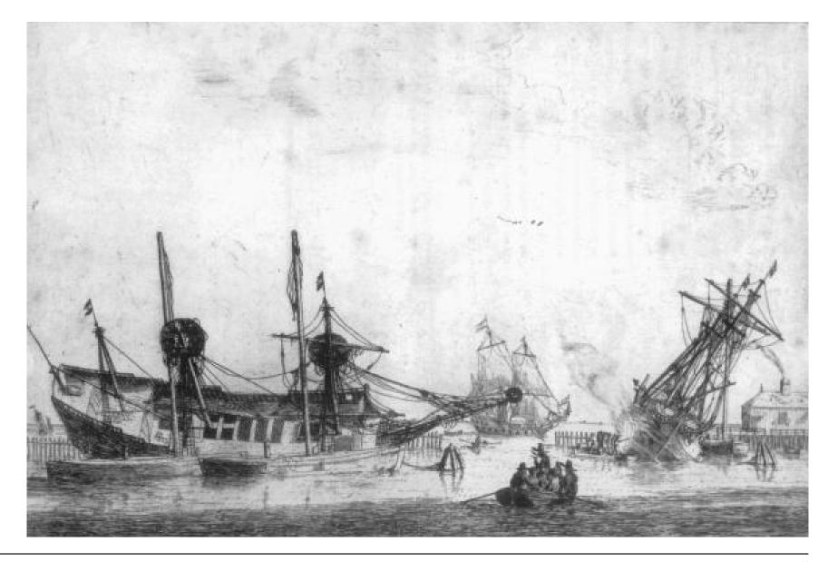
Two vessels careened for caulking the hull, in foreground rowing-boat
